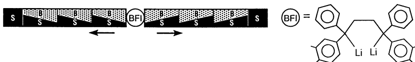
Figure 1. Synthesis routes to Styroflex. The bars indicate the chemical composition along the polymer chain. The light gray areas within the bars symbolize butadiene, the dark areas styrene.
